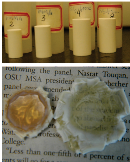
Figure 11. (Top) Samples before compression: (left two) X-Si-1-PMMA , \rho_b = 0.66 \text{ g cm}^{-3} ; (right two) X-Si-1-PS , \rho_b = 0.46 \text{ g cm}^{-3} . (Bottom) Samples after compression: (left) X-Si-1-PMMA , compressed by 86% strain; (right) X-Si-1-PS , compressed by 96% strain.
